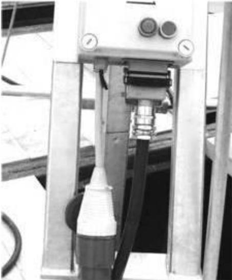
Power supply by means of 5-pole CEE plug-in connection.
